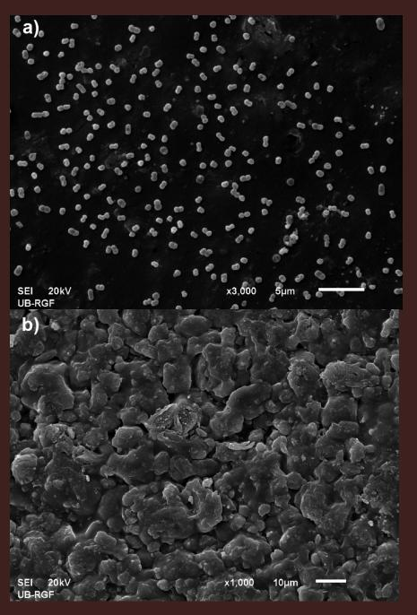
SEM images after 24 h of contact (a) immobilised cells of *A. baumannii* without any sign of biofilm formation on the surface of the Ag-NZ15 composite
